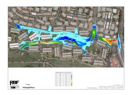
Increasing the capacity of proposed storm drains will also be evaluated for impacts to regional facilities. Based on existing condition flows tributary to each regional facility (i.e. surface and subsurface), proposed condition hydrology and hydraulics will be calculated to ensure no negative impacts to existing regional facilities occur.
